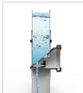
THE K-VALVE 100MM PLUG RELIEVES THE WATER TEST THROUGH THE QUARTER TURN RELIEF VALVE
